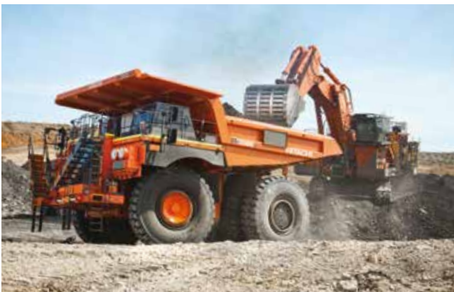
EH dump trucks and EX ultra-large excavators
