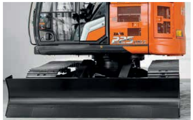
The ultra-short swing radius and optional dozer blade of the ZX225US-7 increase versatility.
