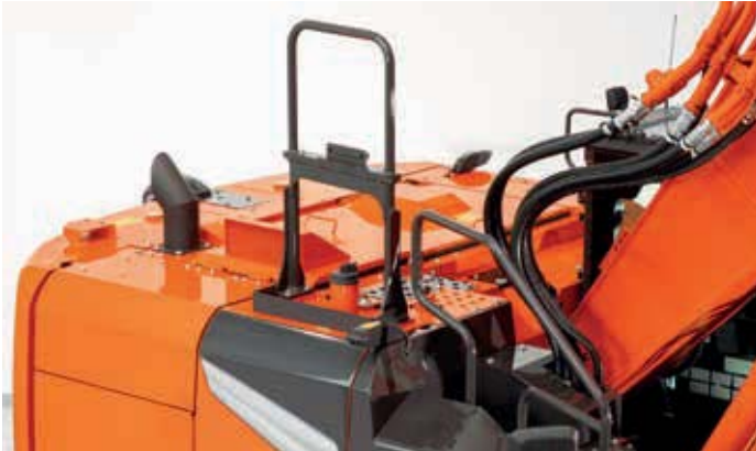
New hand rail on the ZX225US/USR-7 is retractable for easy transport.
