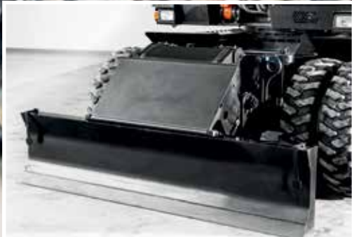
Large blade cylinder cover offers greater protection.
