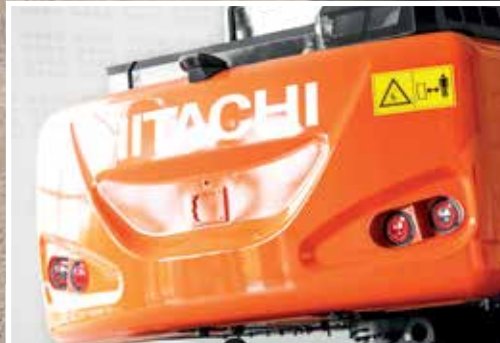
LED tail lights are easily maintained.
