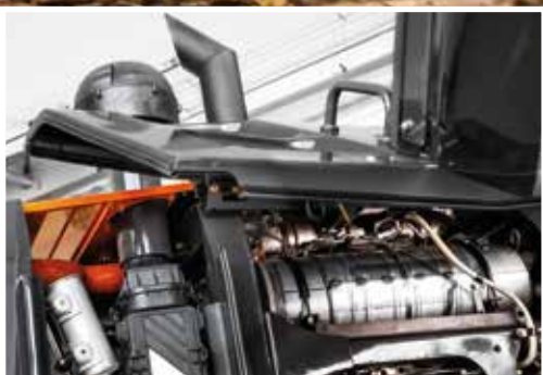
The SCR system reduces emissions.
