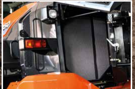
Anti-clogging radiators enhance durability.
