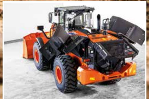
Easy access for maintenance from ground level.
