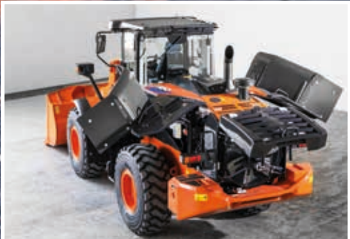
Easy access for maintenance from ground level.
