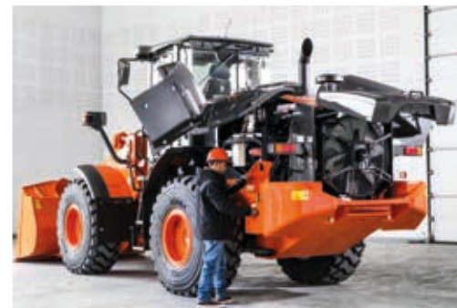
Easy access to the engine compartment.
