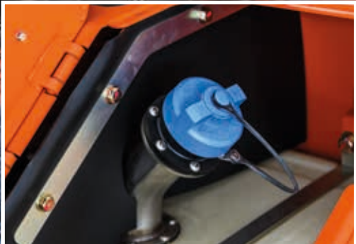
Urea is injected into the exhaust gas to reduce emissions.
