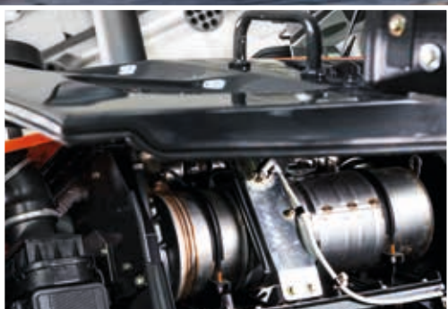
The SCR system reduces emissions.
