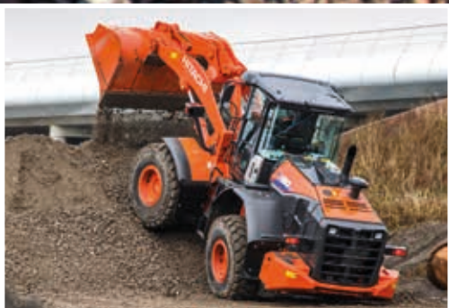
The optional belly guard provides added protection.
